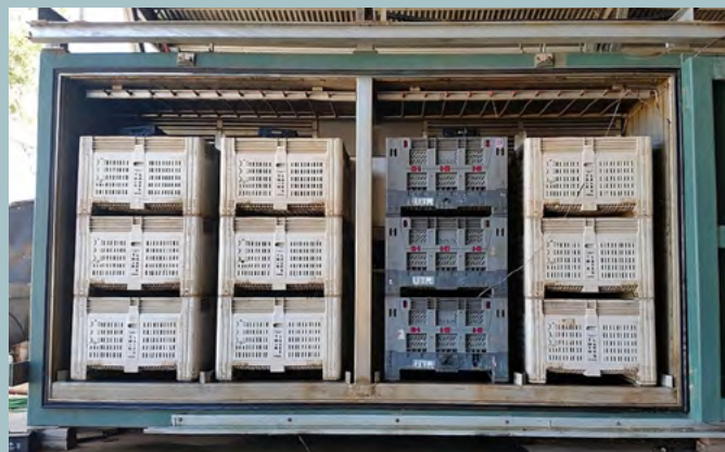
A vacuum-hydro cooler combines vacuum cooling and hydrocooling technologies. The machine sprays the broccoli with water as the vacuum turns the crop moisture into vapor to quickly cool it. Photo from Postharvest Management of Vegetables
