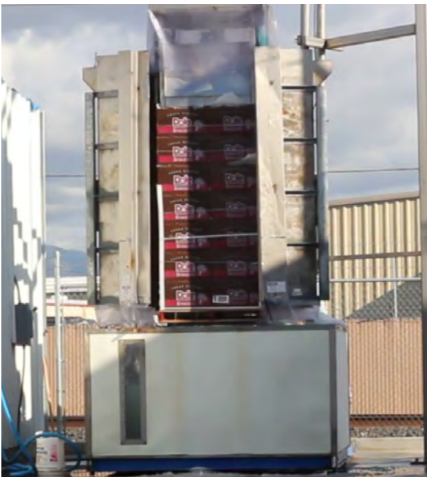
An ice slusher encloses pallets of broccoli to inject a slurry of water and ice. Photo from Eastern Broccoli Project
